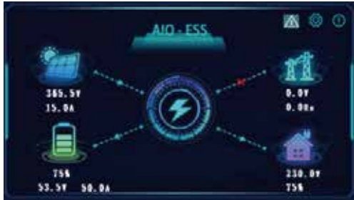
▲ The solar power will supply the load and charge the battery.
