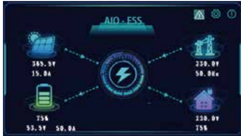
▲ AC Input and solar charging.
