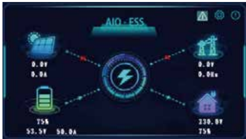
▲ Battery power will supply the load only .
