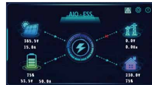
▲ Batteries and solar power supply the load .
