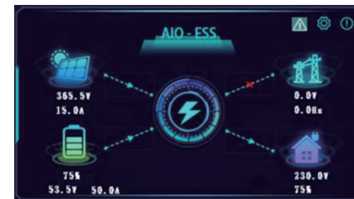
▲ Batteries and solar power supply the load .
