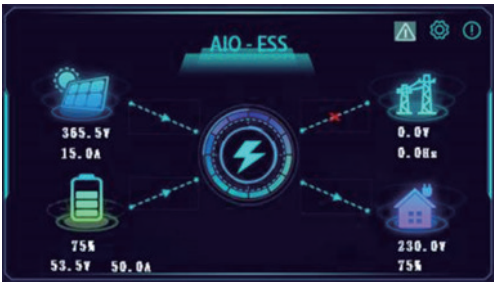
▲ Batteries and solar power supply the load .
